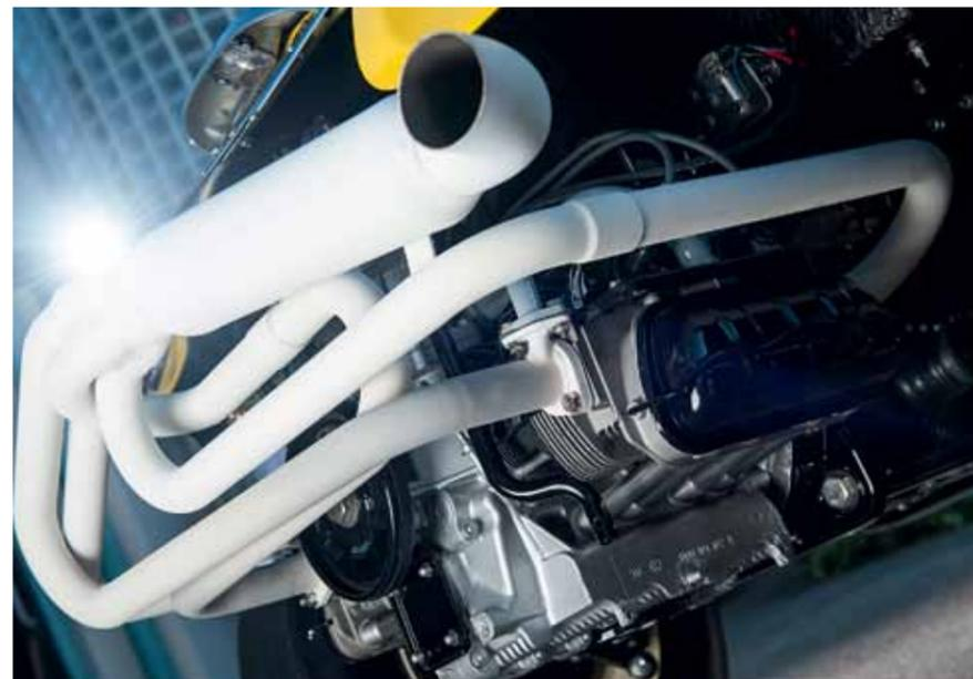
▲ Engine is based on an early '60's 1200 single port, but fitted with a period big bore kit so it now displaces 1384cc. It's basically stock, save for a 1500cc carb, smartened-up tinware and a Bus oil bath air filter.
