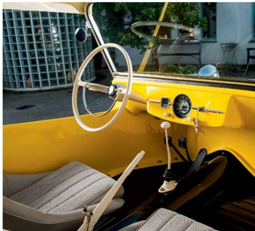
▲ The deceptively simple looking dash belies the amount of work, or "fannying about", as Mark put it, that went into modifying dash trims to sit straight, and to continue the line between the speedo and the fuel gauge.
