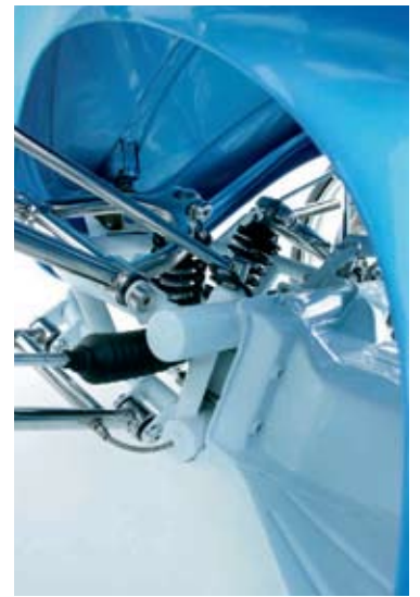
▲ Rear view of front suspension gives a better idea of how it all bolts to the pan
