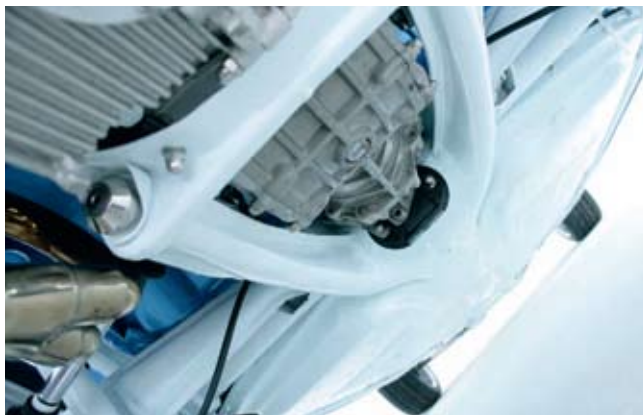
▲ Allen-head machined bolt caps have been used nearly everywhere and where not, they're stainless acorn head nuts. That's attention to detail
