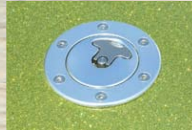
▲ Flush-mounted aero-style filler cap goes well with the Center Line wheels. With more Sixties wheels, you'd want a flip-top cap
