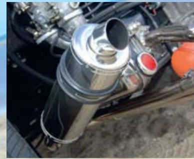
▲ High-quality BAS exhaust has been modified with dual superbike cans. Note the discreet reflectors to keep things legal
