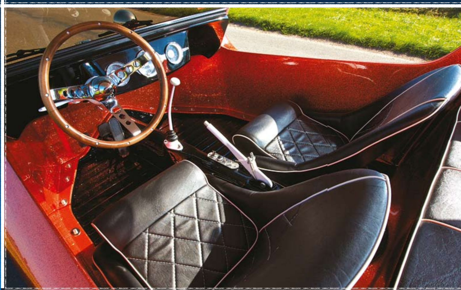
▲ The seats in Steve's Buggy were re-trimmed in black vinyl with diamond pleat inserts and white piping by Brockwells in King's Lynn. That steering wheel is a Grant, of course.
